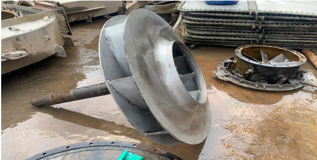
Fig 2.1(a) PA Fan impeller before balancing
