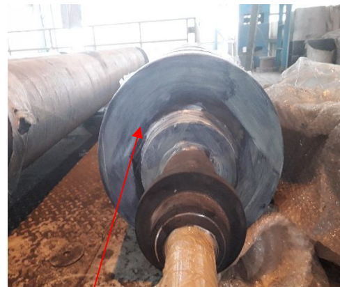
New Rollers ready for installation
