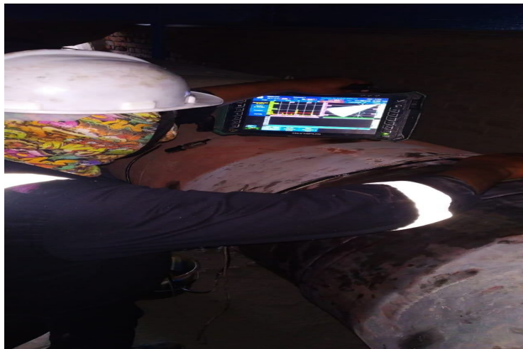
Figure 5: PAUT completed joints
