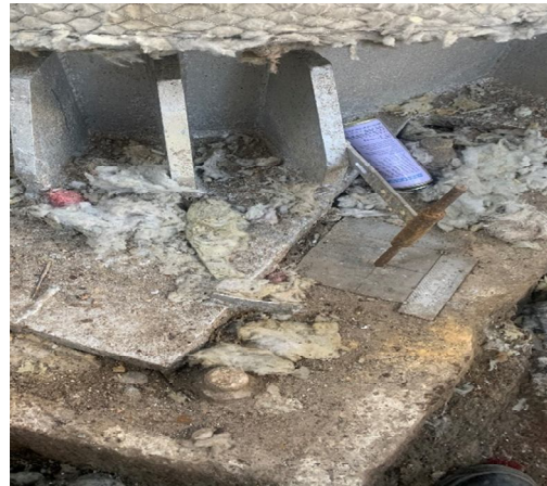
Fig 1.5(a) Arrangement for boiler thermal expansion measurement
