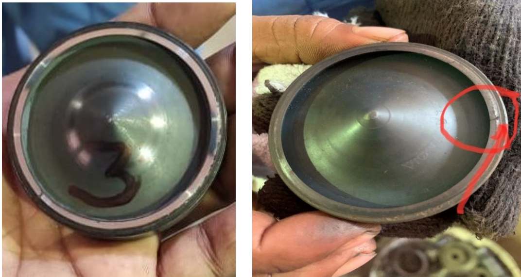
Fig 2.3(b) Scratch on Steam Drum& SH1 Safety valve disc
