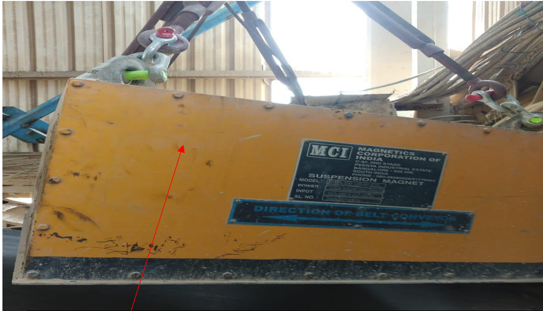
NEW ELECTRO-MAGNET PROVIDED IN THE DRIVE END OF THE CONVEYOR TO REMOVE FOREIGN METALLIC PARTICLES
