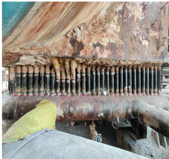
Boiler bypass nozzle top portion badly damaged which is replaced with new one.
