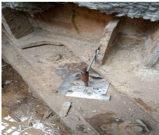
Fig 1.5(a) Arrangement for boiler thermal expansion measurement
