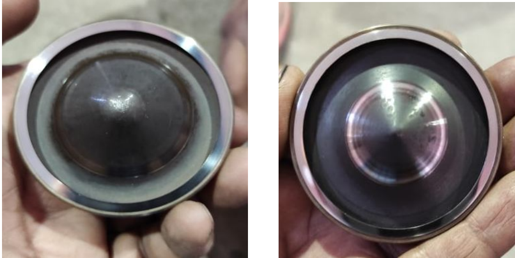
Fig2.3(a) disc insert after lapping
