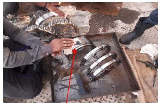
New Bearing ready for installation
