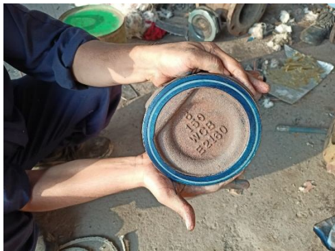
Blue matching of valve disc
