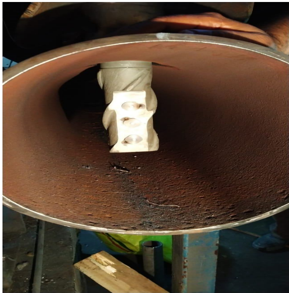
Figure 3: Nozzles for desuperheating
