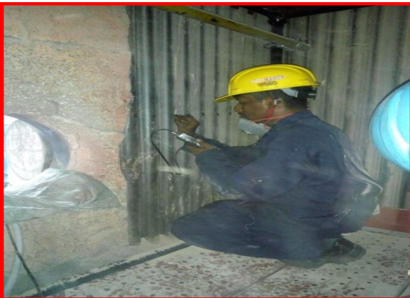
Thickness measurement carried out at various pr.parts in boiler
